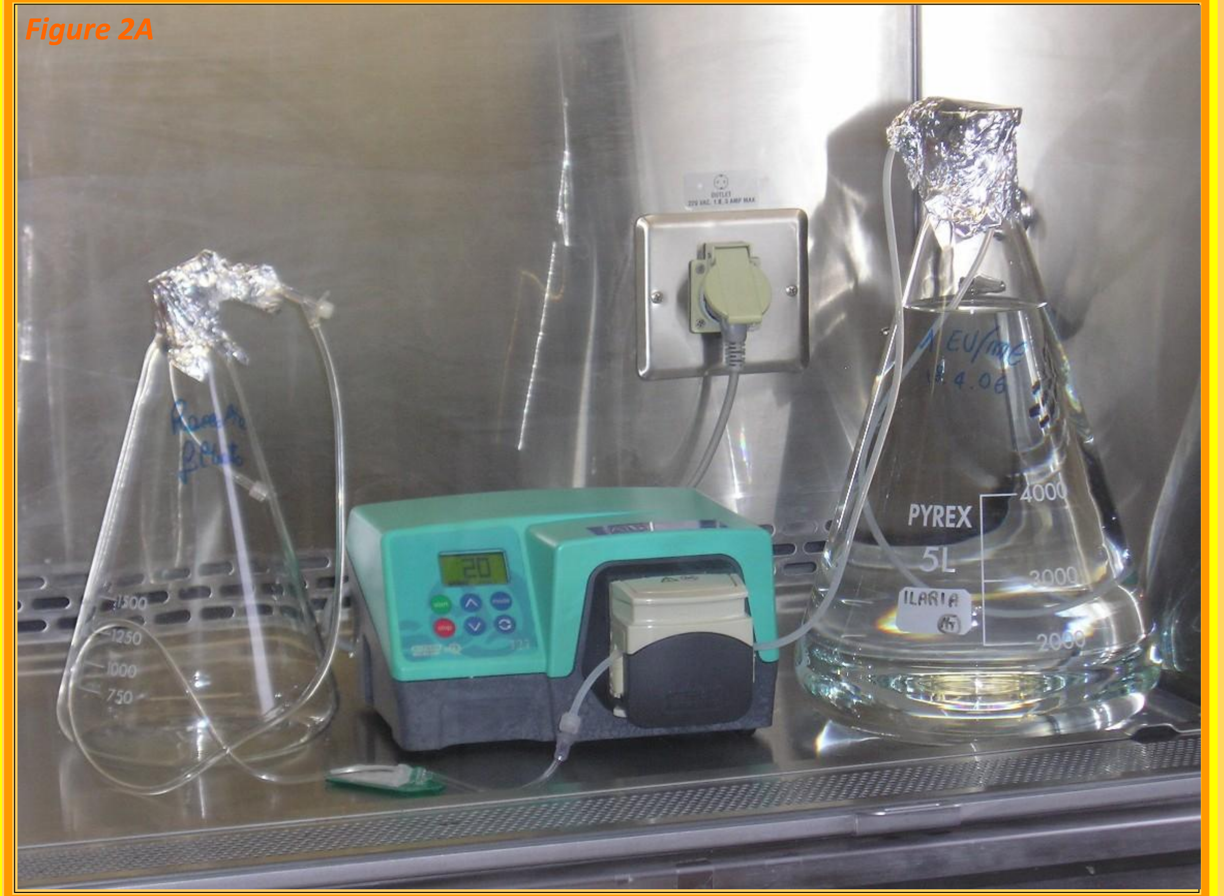
Figure 2: Apparatus used to carry out the test: A infusion pump was used to challenge every tubing set, and so every filter, with the 1 EU/ml CSE solution, as we illustrated in figure 2A and as we draw in figure 2B. Samples of filtrate fluid (FF) and challenge solution (CS) were collected after 0, 8, 24, 48, 72 and 96 hours of flow through the filter. The samples were tested for endotoxin concentration with LAL test gel-clot method.
